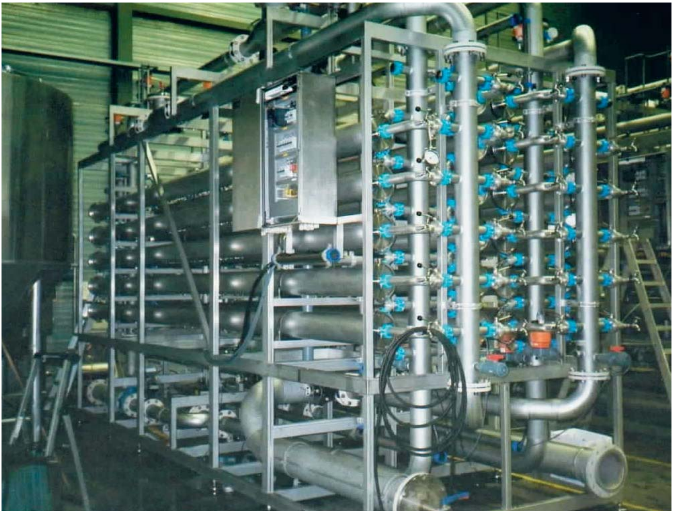
Norit primary membrane unit before leaving factory in Holland (courtesy Black & Veatch)
