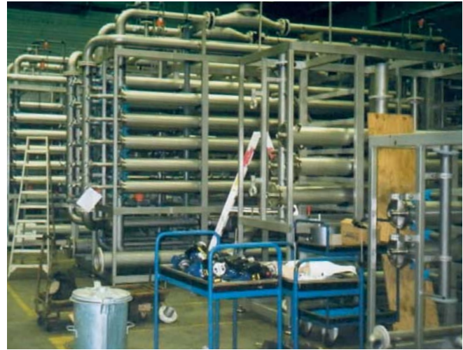
Norit primary membrane units (secondary in foreground) before leaving factory in Holland (courtesy Black & Veatch)
