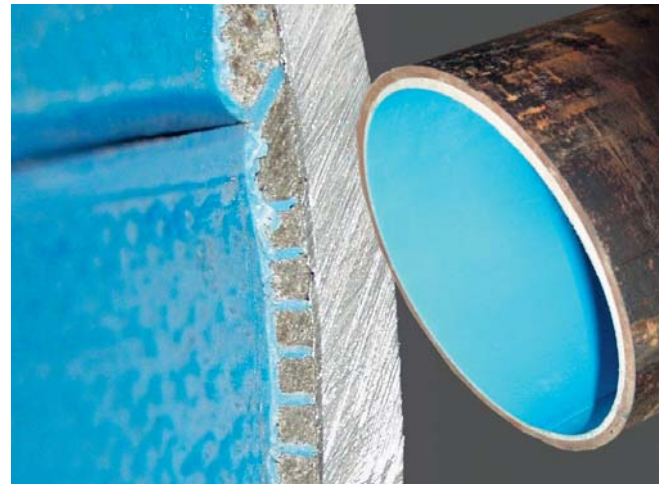
PE Liner prepared for insertion (courtesy Pipeway Ltd)
